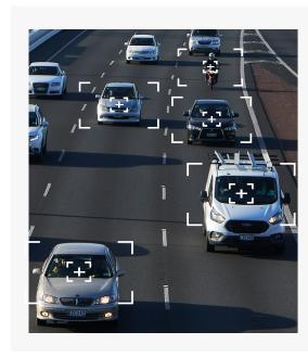
The use of cameras in traffic may have a preventive effect and enhance road safety. With camera solutions from SWARCO you can also carry out measurements of various vehicles and persons over specified distances, for example speed information, queues and congestions, as well as counting and tracking specific objects.
