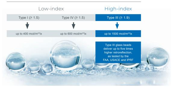
The only difference between type I and IV beads is their size, which also influences their retroreflective values. Type I beads reach up to 400 mcd/m²\*lx. Type IV glass beads are larger than type I beads, with retroreflective values reaching up to 600 mcd/m²\*lx. Type III glass beads are high-index beads. These have better optical properties and significantly higher retroreflective values of up to 1500 mcd/m²\*lx because they are made from special high-grade glass.
