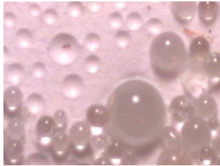
Example of craters caused by beads loss
