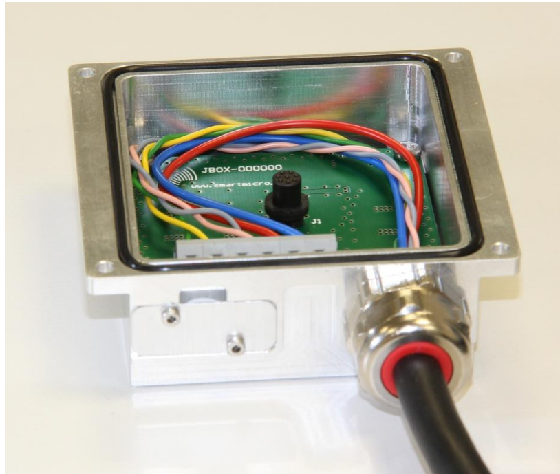
Figure 1: Junction Box RD_Caiman_JB_36 with attached Lapp cable
