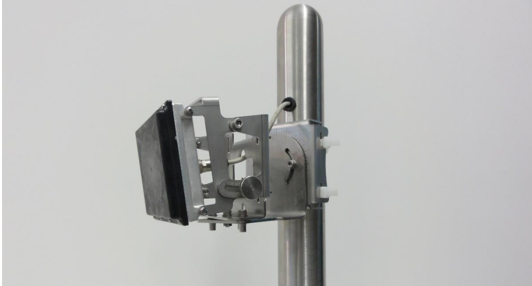
Figure 12: BFW_Caiman_36A attached to pole using straps, straight orientation
