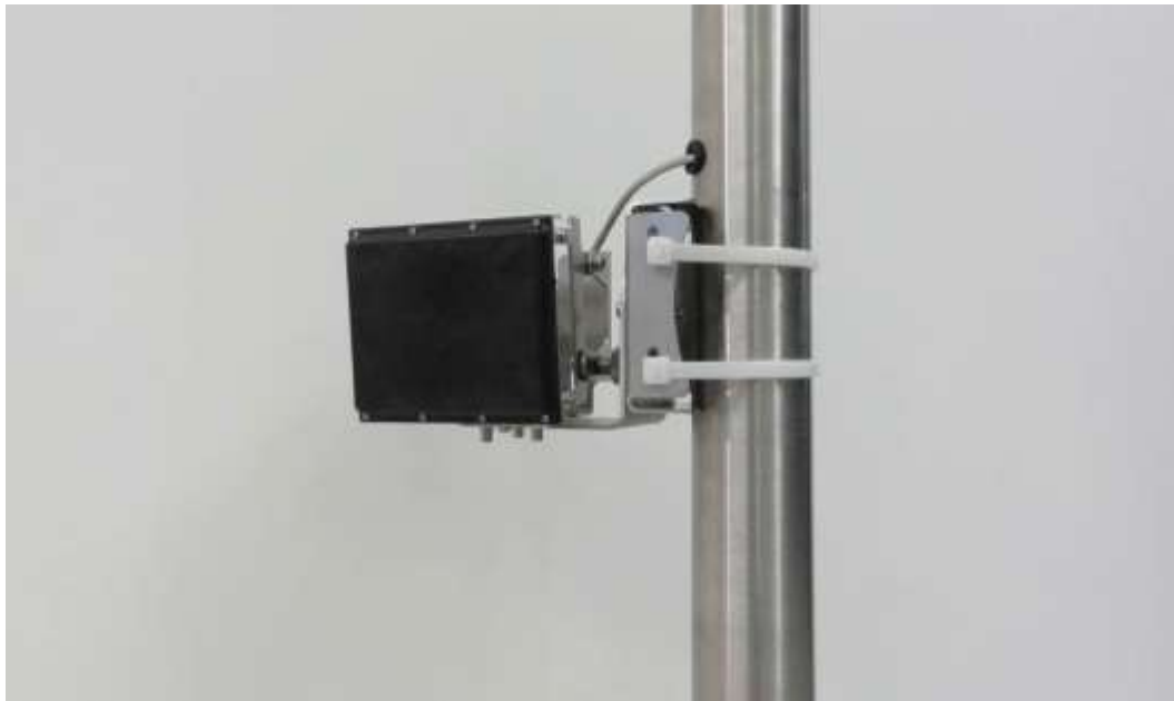
Figure 15: BFW_Caiman_36A attached to pole using straps, right angled orientation
