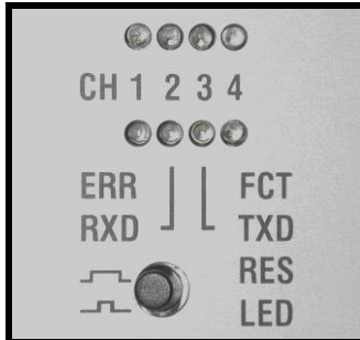
Figure 4: LEDs and pushbuttons at front panel of SW2224
