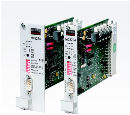
Figure 1: Front view of MC2224 (width 8 and 4 TE)
