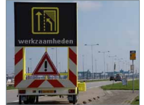
trailer mounted ECO LED mobile variable message sign, full matrix, full color RGB, powered by solar panels, GPRS/GPS communication
