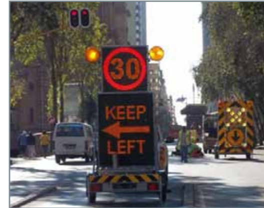
trailer mounted LED mobile variable message sign, full matrix, upper board bi-color red/yellow, lower board mono-color yellow, powered by diesel generator with PDA control unit
