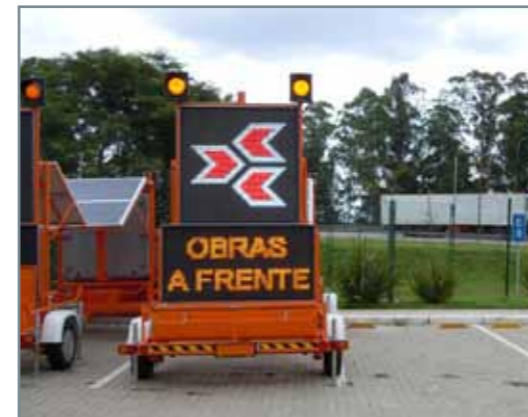
trailer mounted LED mobile variable message sign, full matrix, upper board full color RGB, lower board mono-color yellow, powered by solar panels
