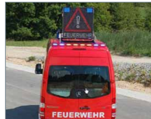
rooftop mounted LED mobile variable message sign, full matrix, full color RGB, powered by batteries with PDA control unit
