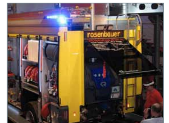
vehicle integrated LED mobile variable message sign, full matrix, mono-color, communication Interface: CAN, protocol: CANopen
