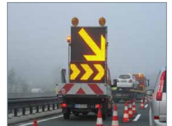
truck mounted LED mobile variable message sign, full matrix, upper board bi-color red/yellow, lower board mono-color yellow, powered by batteries with PDA control unit
