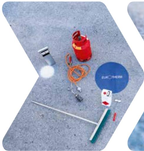
Equipment: Torch, broom, piece of chalk and drop-on material. Use a primer if necessary.
