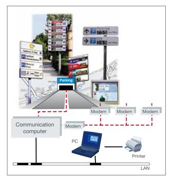
The system is automatically controlled, monitored and if necessary, also manually adjusted by means of a user-friendly user interface at the communication centre.
