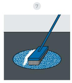
Clean the marking with a broom and use a sharp object to check that it is securely adhered. It can be walked and driven over after just a few minutes.
