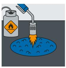
Use the torch to heat the entire surface of SWARCO PREFORMED until it starts to bubble.
