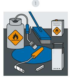
Equipment: Torch, broom, piece of chalk and drop-on material. Use a primer if necessary.
