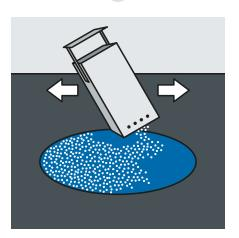
Apply the drop-on beads to SWARCO PREFORMED.
