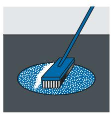
Clean the marking with a broom and use a sharp object to check that it is securely adhered. It can be driven over after just a few minutes.
