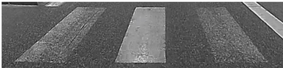
Fig. 2. Exemplary area (crossing B) after 3 years and 23.0 million weight-adjusted vehicle passes: circa 43% marking loss.
