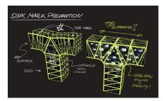
In plastics processing, the use of glass beads reduce sink marks.
