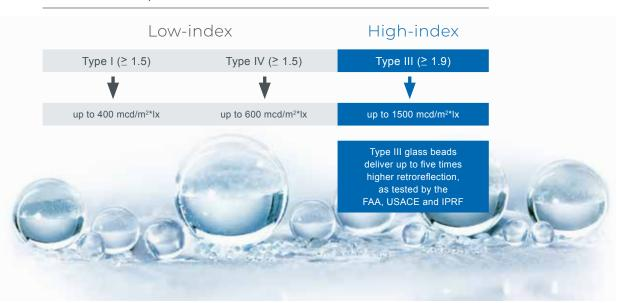
The only difference between type I and IV beads is their size, which also influences their retroreflective values. Type I beads reach up to 400 mcd/m²\*Ix. Type IV glass beads are larger than type I beads, with retroreflective values reaching up to 600 mcd/m²\*Ix. Type III glass beads are high-index beads. These have better optical properties and significantly higher retroreflective values of up to 1500 mcd/m²\*Ix because they are made from special high-grade glass.
