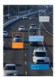
The use of cameras in traffic may have a preventive effect and enhance road safety. With camera solutions from SWARCO you can also carry out measurements of various vehicles and persons over specified distances, for example speed information, queues and congestions, as well as counting and tracking specific objects.
